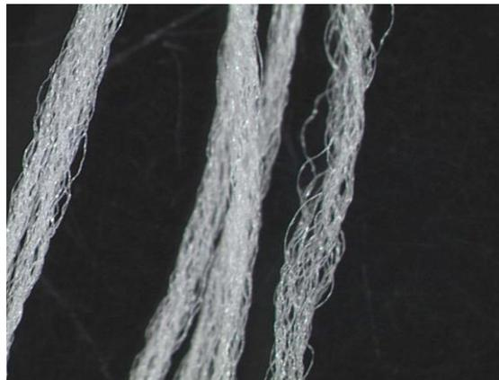
**Figure 5: Polyester woven yarn to manufacture the graft, since it has high porosity and can withstand greater radial force.**
