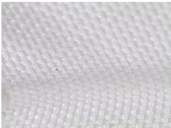
**Figure 4: Polyester woven yarn to manufacture the graft, since it has high porosity and can withstand greater radial force.**
